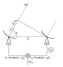
For a finite bandwidth and non-zero delay, the fringe amplitude is attenuated by the factor  $\operatorname{sinc}(\Delta \nu \tau_g)$ . This can be compensated in any one direction  $\hat{s}_0$ , that is called the delay center by using a compensating delay  $\tau_0 \approx \tau_{\rm g}$  (usually digital).
