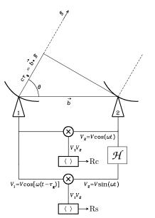
The sine part of the correlator can be implemented simply by introducing  $90^{\circ}$  phase shift to the second branch of the correlator. The  $90^{\circ}$  phase shift is mathematically the *Hilbert transform*  $\mathcal{H}$  of the signal.
