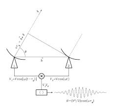
After multiplication the product of the antenna voltages is averaged with a timescale of typically seconds, so that the term  $\cos(2\omega t - \omega \tau_{\rm g})$  averages out.
