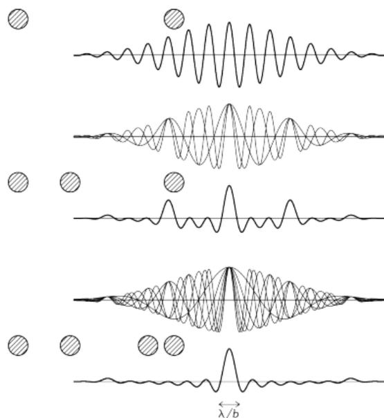
Isotropic antenna elements would fill the sky with a sinusoid response. Individual responses of (real world) directive antenna elements are multiplied with the sinusoid, result is a 'sinusoid pulse' pattern.
