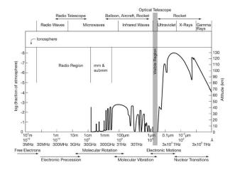
Atmosphere is reasonably transparent from about 15 MHz to 1.5 THz. The graph shows the altitude where the radiation is attenuated by half.
