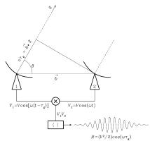
$$\frac{d\phi}{d\theta} = \frac{\omega}{c}b\sin\theta = 2\pi\left(\frac{b\sin\theta}{\lambda}\right) \quad (9)$$
