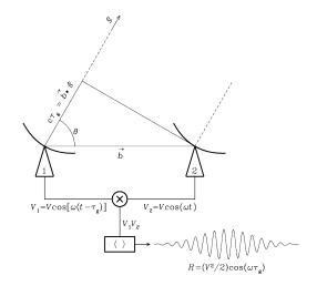
At frequency  $u = \omega/(2\pi)$  the signals from antennas are
