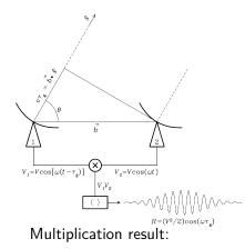
After multiplication the product is averaged with a timescale of typically seconds), so that the term  $\cos(2\omega t - \omega \tau_g)$  averages out.
