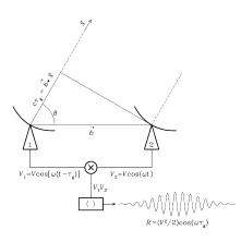
The correlation result  $\left(\frac{V^2}{2}\right)\cos(\omega\tau_g)$  varies sinusoidally because the source direction is slowly changing (earth rotation). These sinusoids are called *fringes. Fringe phase* is
