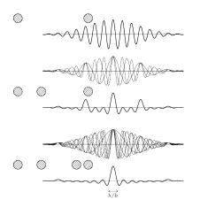
Isotropic antenna elements would fill the sky with a sinusoid response. Individual responses of (real world) directive antenna elements are multiplied with the sinusoid, result is a 'sinusoid pulse' pattern.
