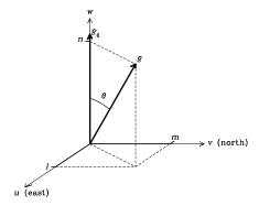
The (u, v, w) coordinate system is used to describe any baseline vector  $\vec{b}$  in three dimensions. The *w*-axis points usually to the source  $\hat{s}_0$ . The *u* and *v* axes point east and north and are in wavelenghts.
